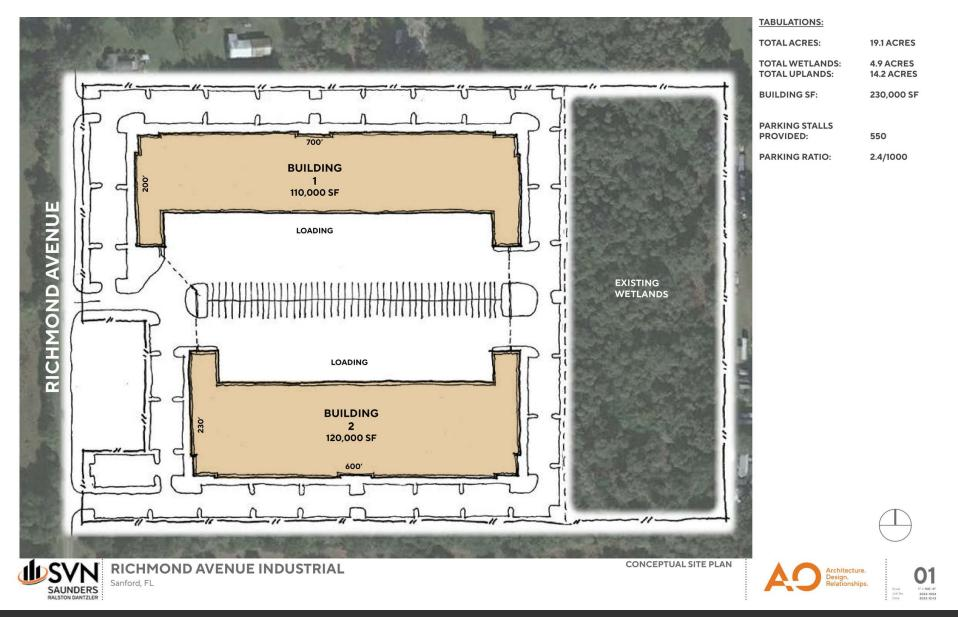
Conceptual Site Plan with Two-Rear Load Configuration Warehouse buildings.
